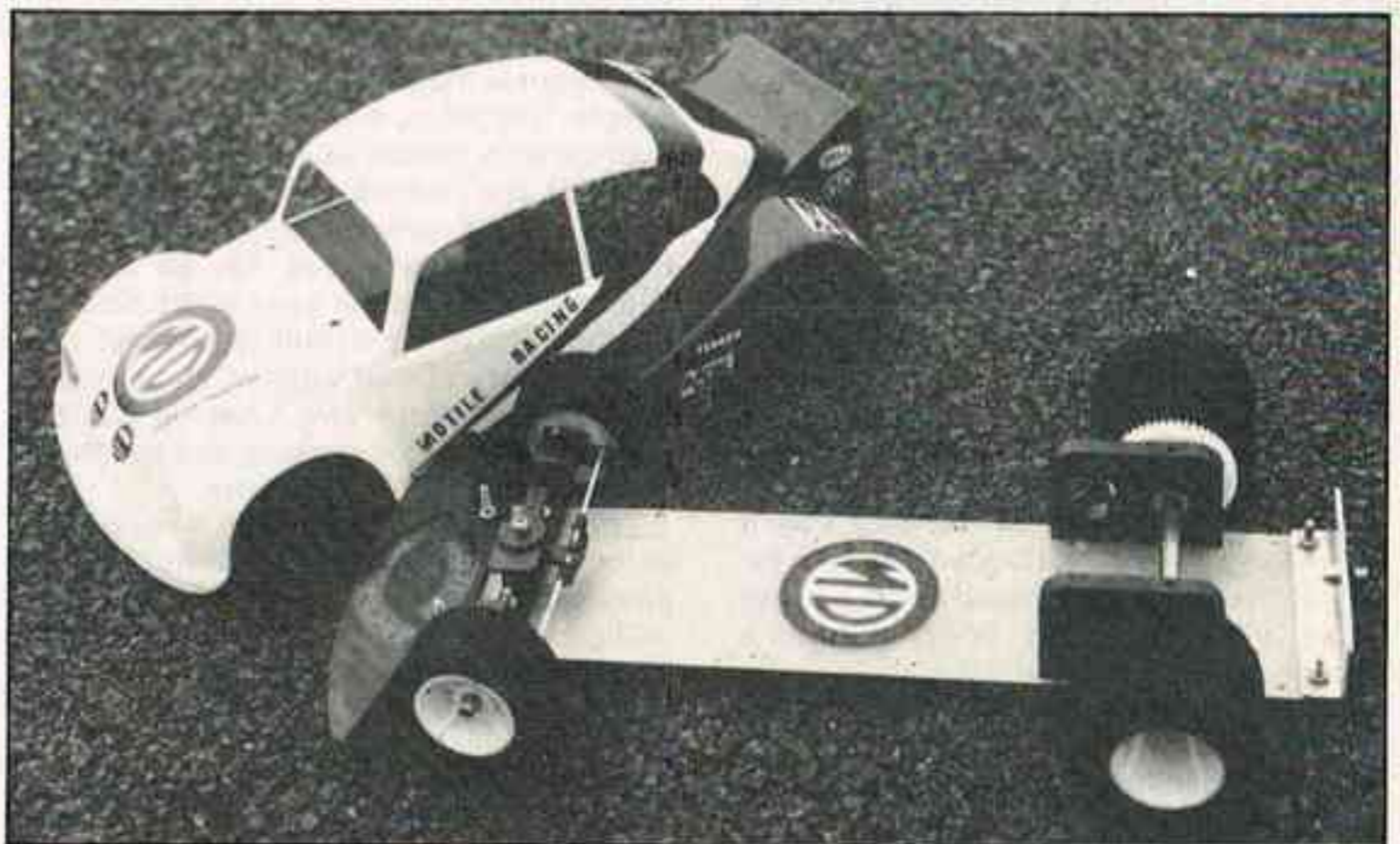
Above, the rolling chassis and the Beetle body shell, this shell has been spray painted using normal cellulose car sprays, the shell is ABS plastic and requires the windows and wheel arches cutting away before you paint your Wagon. Below, the Beetle looks like a real flier and it does, but the theme of limited cost racing is what this car is all about, the use of Mini Stock components ensures the continuation of low cost competitive racing, either on the Oval or circuit.
