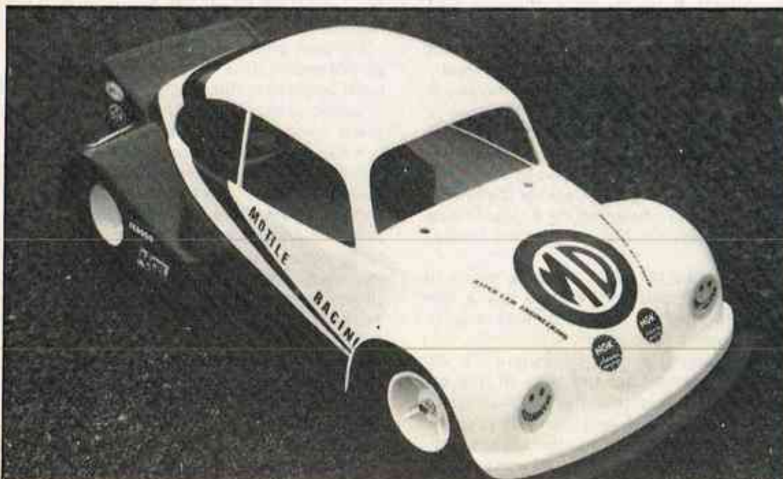
Above, the rolling chassis and the Beetle body shell, this shell has been spray painted using normal cellulose car sprays, the shell is ABS plastic and requires the windows and wheel arches cutting away before you paint your Wagon. Below, the Beetle looks like a real flier and it does, but the theme of limited cost racing is what this car is all about, the use of Mini Stock components ensures the continuation of low cost competitive racing, either on the Oval or circuit.
