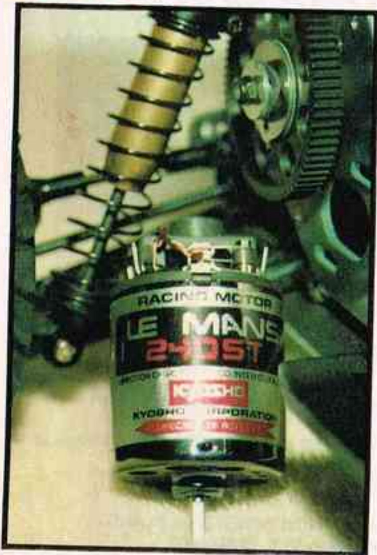
Le Mans 240ST motor comes standard on the 'Mid' with a three step mechanical speed controller.
