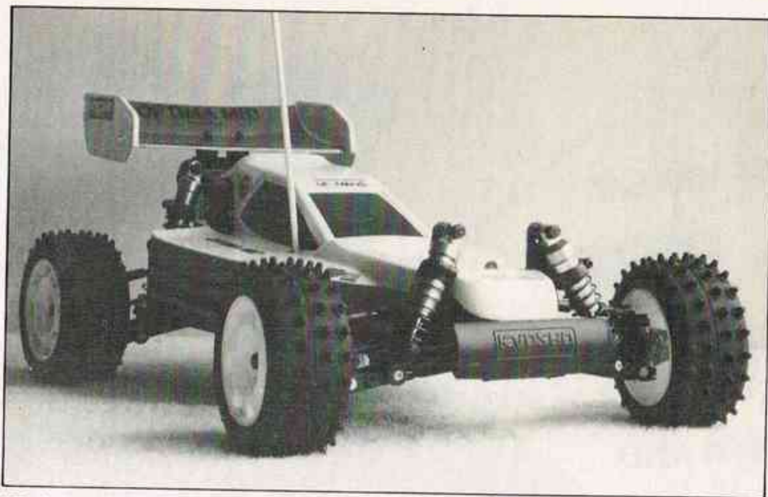
"Turbo" in its original paint scheme. The shock absorbers are mounted more vertically than on the original Optima.
