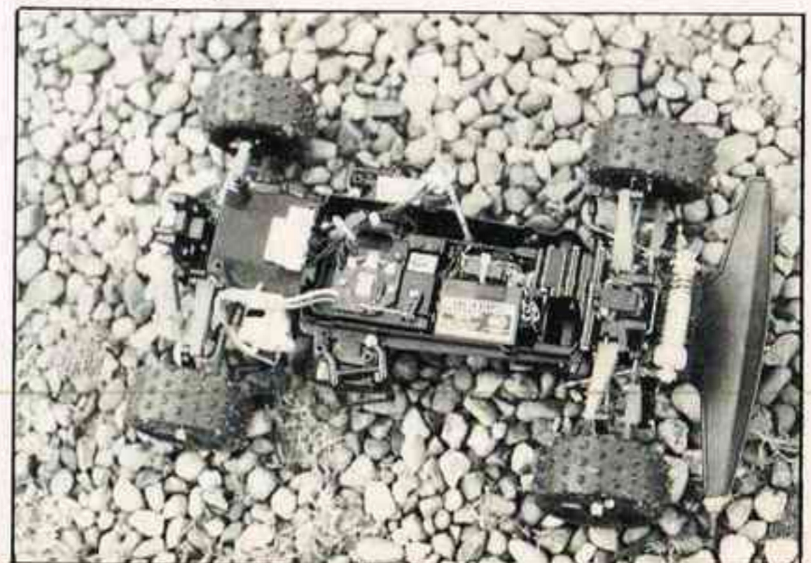
The bare bones, the swinging battery keeper can be clearly seen in this shot.
