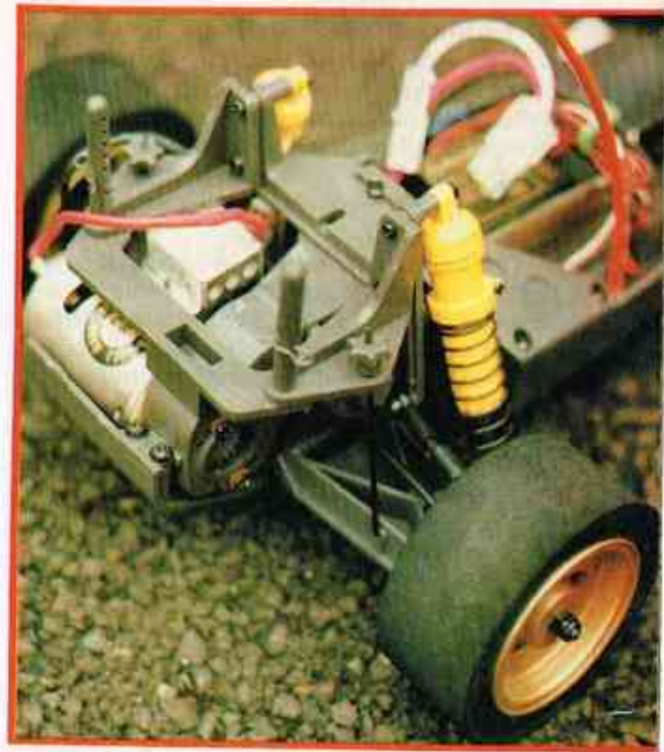
Above and left, clearly shown in these photos are the suspension ride height adjustment system. Left the Thunderbird comes complete with two sets of tyres, on and off road.
